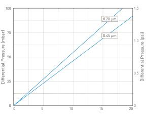
Flow (L / min) for liquid @ 20 °C and 1 cp 10  $\!\!\!^{"}$  module
